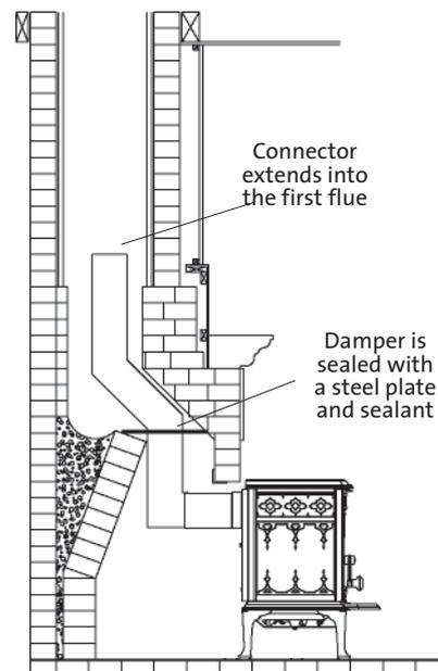
Figure 7. Hearthmount Installation.
